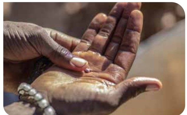
A small piece of gold emerges after mercury is used to separate gold particles from the ore powder at a small-scale gold mine, Zimbabwe.
