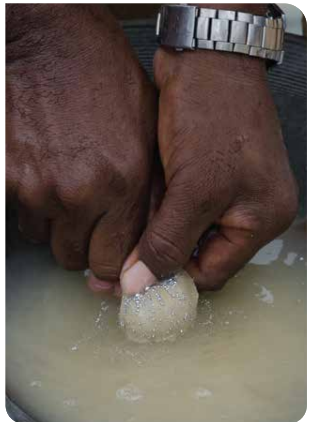
Miner uses mercury to separate out the gold from waste minerals, Guyana.
