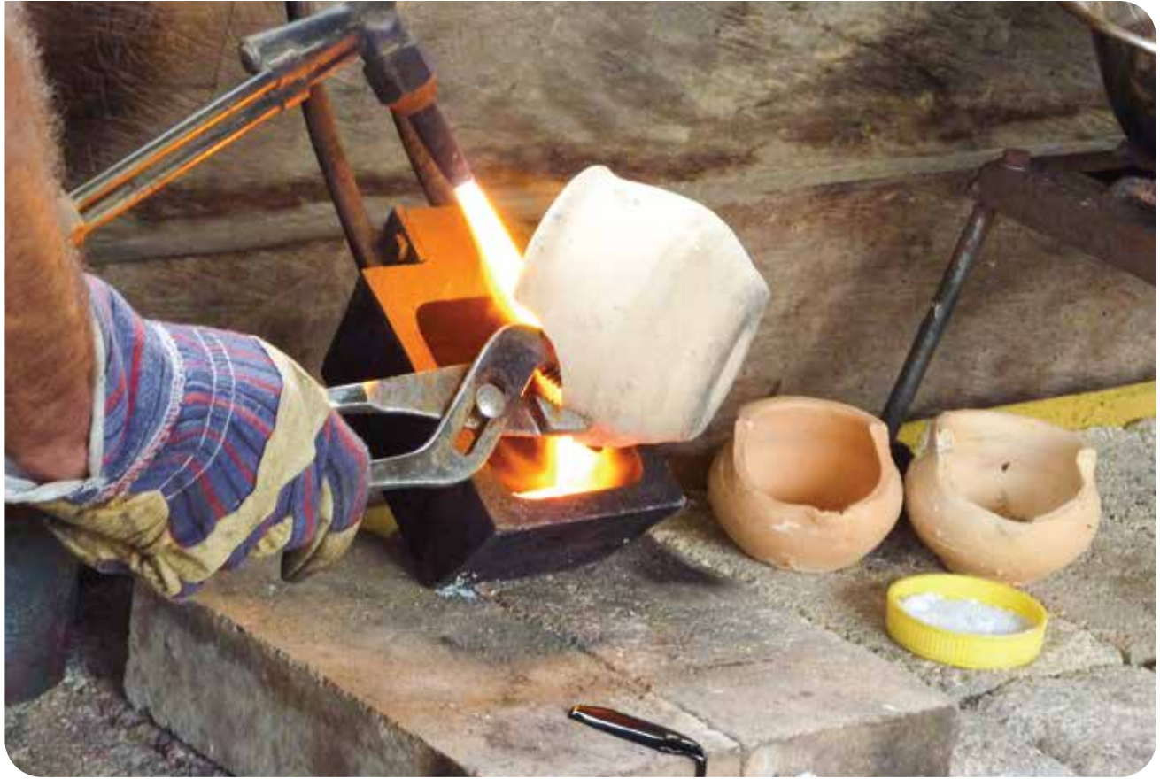
The concentrated gold charge is heated with Borax before being poured into a Gold bar, Guyana.
